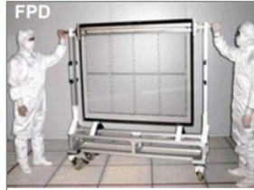
Exposure Process used to Create a TFT Circuit Pattern
